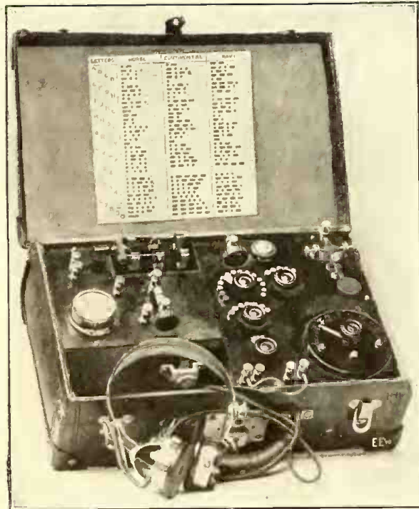
Fig. 1, Appearance of Completed Radio Sending and Receiving Set. Sending Range 3 to 5 Miles. Has Received 300 Miles and is Capable of Much Finer Work.
