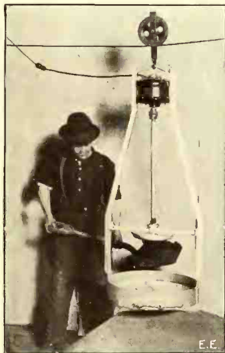
New Motor Driven Riddle for Foundry Work, a Great Time Saver.
